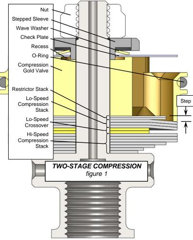
The Restrictor Valving serves a second function. If we increase the diameter, it restricts the flow area of the ports. This increases the damping at high velocities like landing off a jump but can make it harsher on square-edge bumps.
